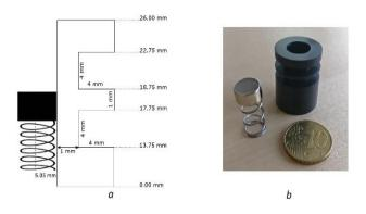
The spring used in the single-spring design is a normal commercially available helical spring made of stainless-steel wire with a diameter of 0,81 mm. The diameter of the spring is 9,14 mm, the length of rest is 15,75 mm, and the spring constant is 2,17 N/mm.
