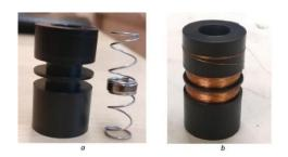
After the first prototype implemented it became aware that a harvester with smaller dimensions with the same power output would be possible to construct, if only one spring with a greater spring constant would be used. The values for the spring and the magnet were recalculated and a new housing was lathed. The housing of the second prototype has dimensions 20,10 mm x 26,00 mm, which is 7,0 mm lower than the first version. The dimensions are shown in figure below on left (a),
